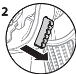
Gun unlocked (gun will spray)
