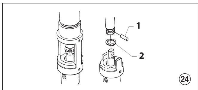
9. Remove the piston rod assembly from the motor/pump block (31).
