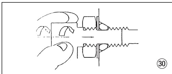
4. Back fitting out no more than one complete turn to align as required.
